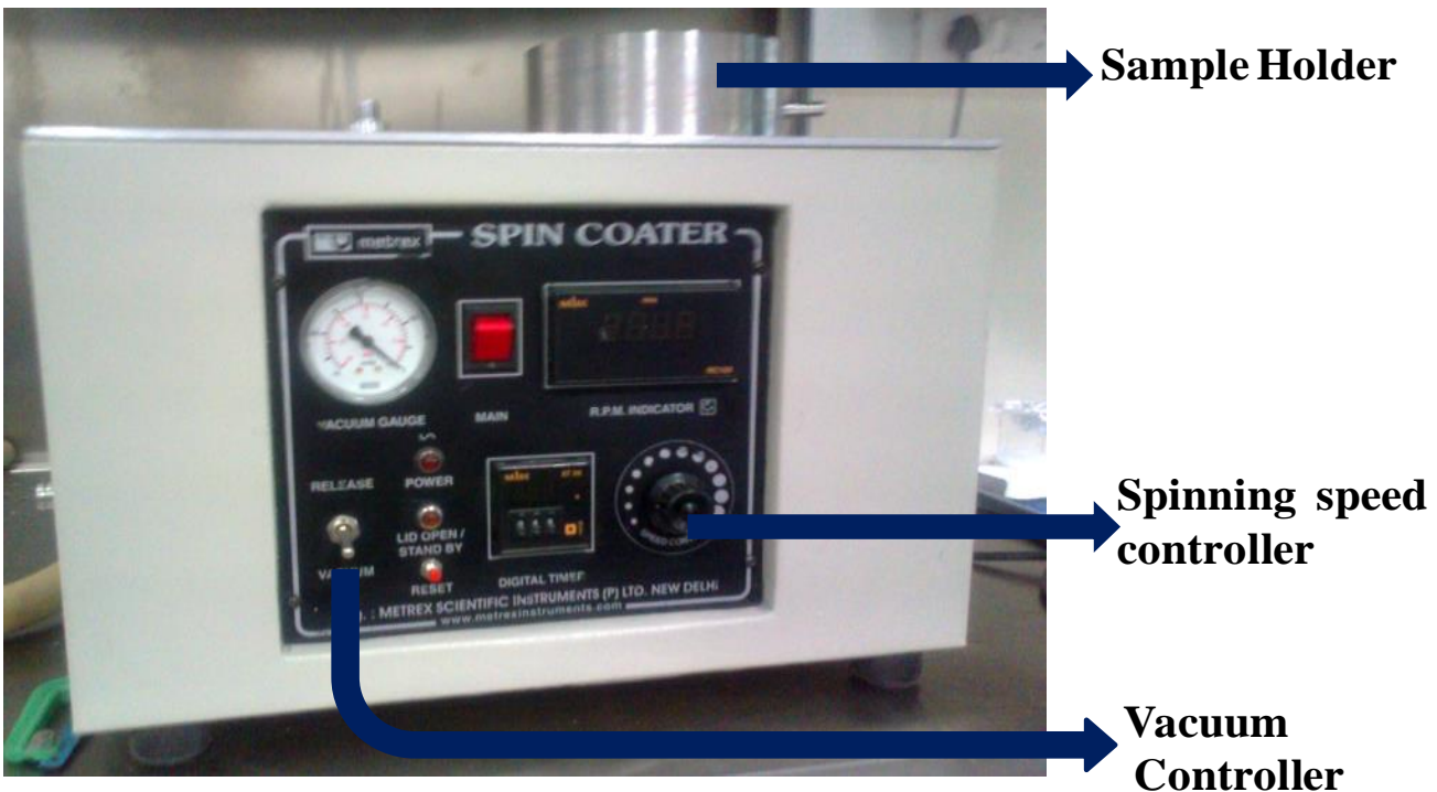
Figure A.1.4: Photograph of spin coater used in the preparation of thin film
