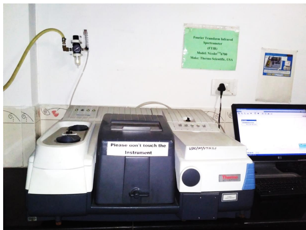
Figure A8 Experimental setup of FTIR spectrophotometer (USIC BBAU Lucknow)
