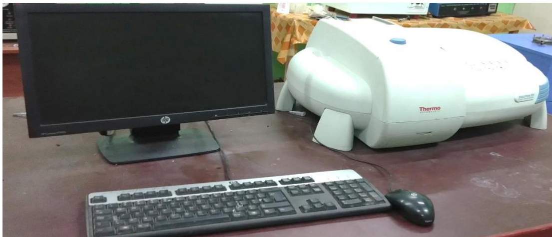
Figure A5 Experimental setup of UV visible spectrometer Evolution 202 (NMSL BBAU Lucknow)
