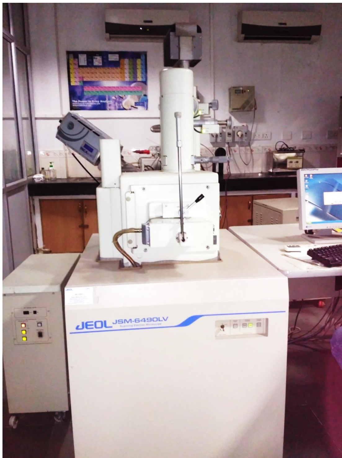
Figure A4 Experimental setup of Scanning Electron Microscope JEOL JSM-6490LV (USIC BBAU Lucknow)
