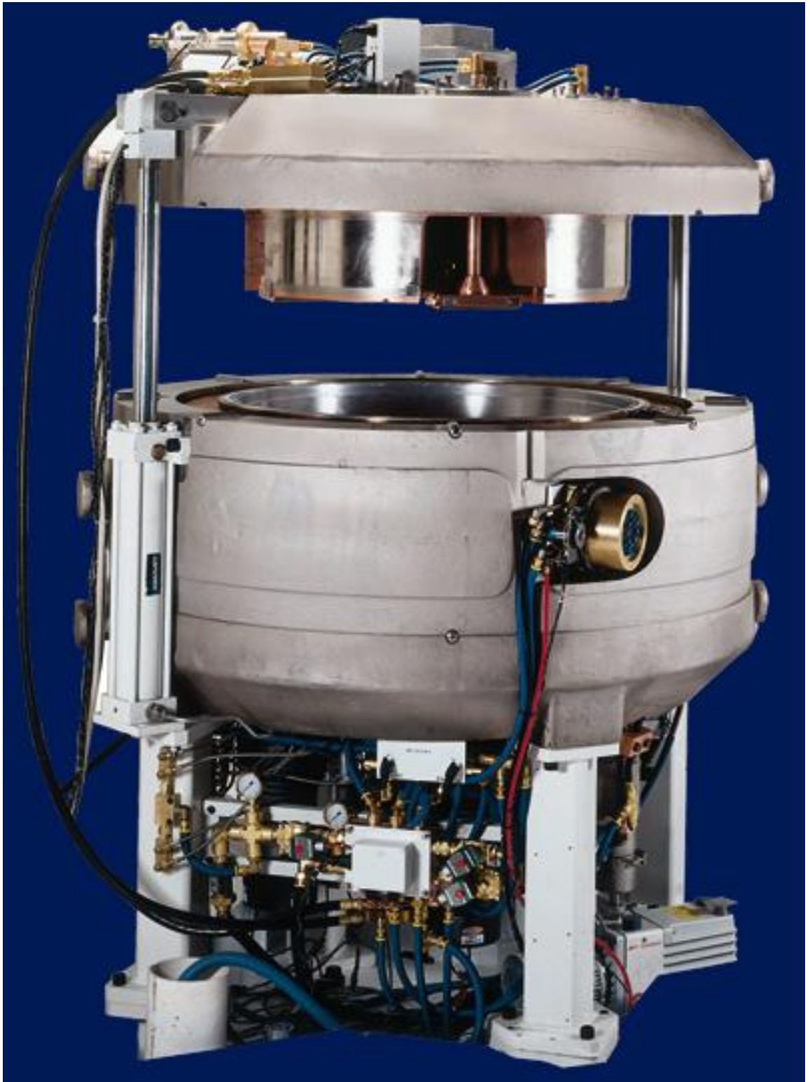
Figure 1.2: Picture of Medical Cyclotron without Shielding (Courtesy Siemens Ltd)
