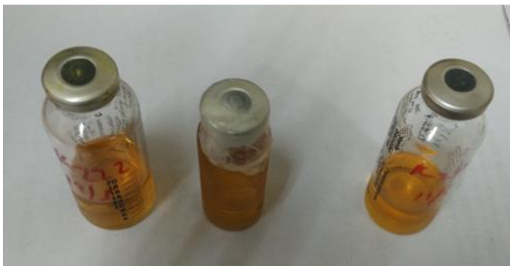
Figure 3.13: Colour of septa Changes when we use bad quality of septa
