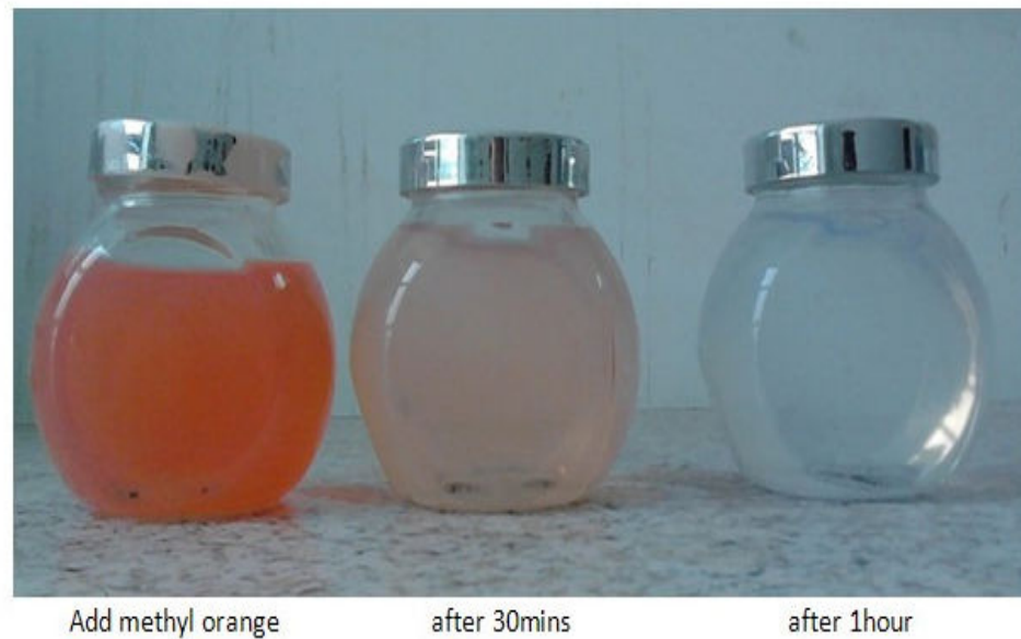
Fig.1.13. Waste water treatment by photodegradation
