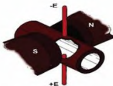
Fig. 1. Pulsed magnetic field generator and cell used in industrial tests.
