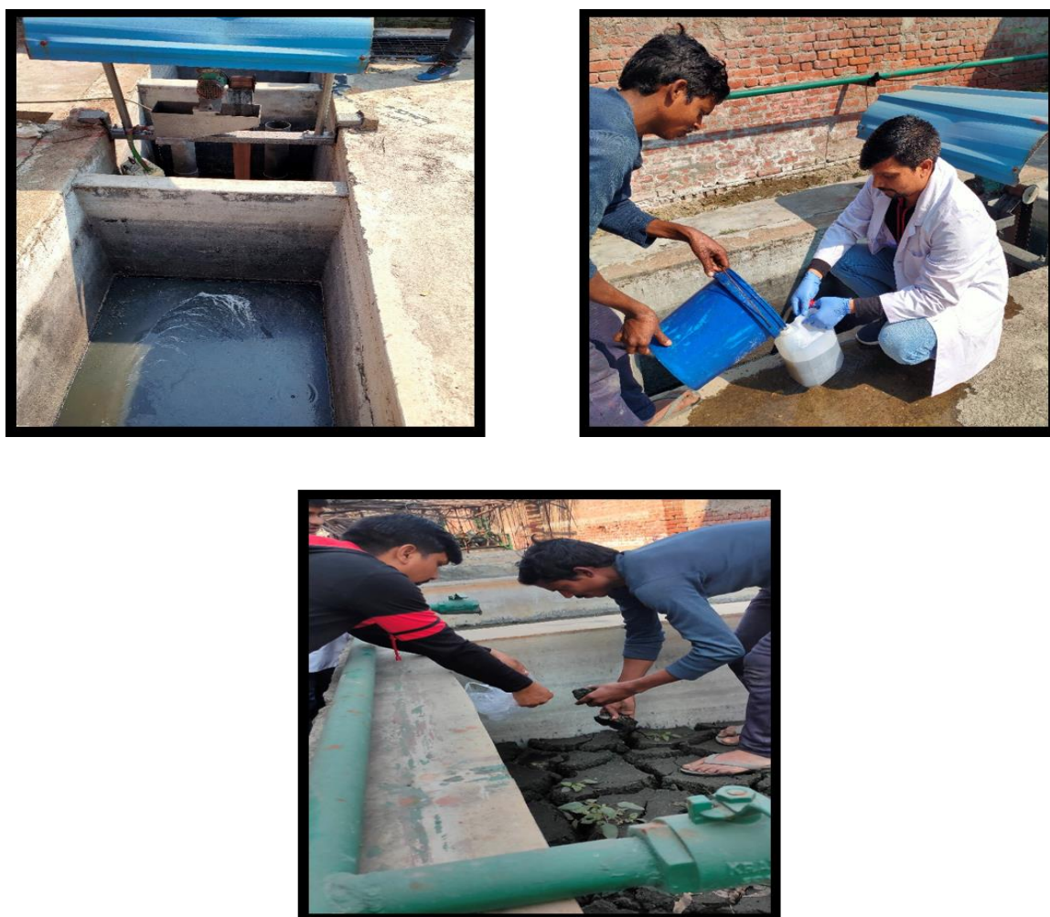
Fig 4.1: Collection of textile wastewater from the outlet of a Handloom Bhandar, Unnao, Uttar Pradesh, India.
