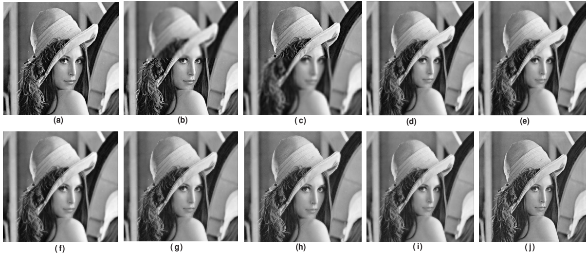
Figure 5: Fusion results for lena image: (a) Reference image (original image); (b) blurred on upper part; (c) blurred on lower part; (d) fused image by DWT; (e) fused image by DWT + PCA; (f) fused image by MSVD; (g) fused image by SWT; (h) fused image by CVT; (i) fused image by NSCT; (j) fused image by proposed scheme.
