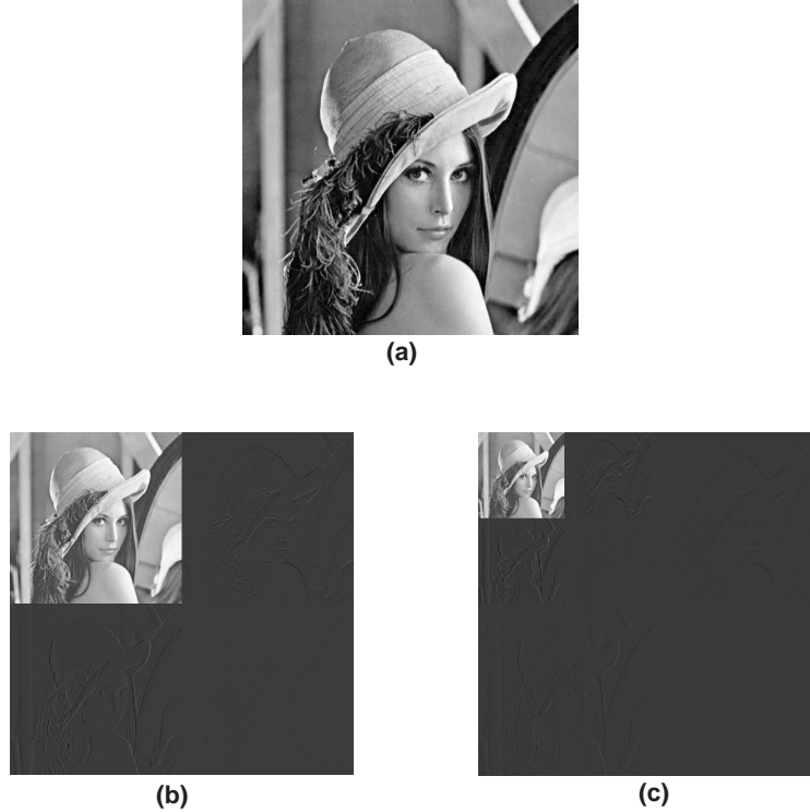
Figure 3.2: DWT decomposition of Lena image. (a) Lena image; (b) first level 2-D DWT decomposition; (c) second level 2-D DWT decomposition.
