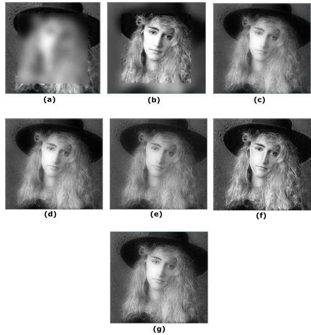
Fig.7. Fusion results for hoed image: (a) middle part blurred; (b) boundary part blurred; (c) fused image by DWT; (d) fused image by PCA; (e) fused image by SWT; (f) fused image CBF; (g) fused image by proposed method.
