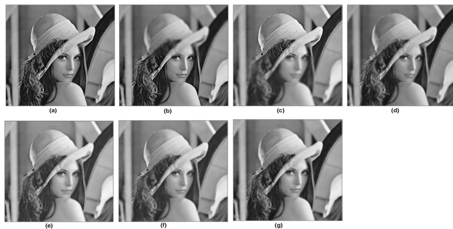
Figure 3.7: Fusion results for lena image. (a) Reference image; (b) upper side blurred image; (c) lower side blurred image; (d) maximum method; (e) minimum method; (f) directive contrast method; (g) G-DWT method.
