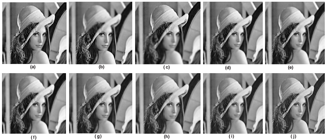
Figure 5.4: Lena image. (a) Reference image (original image); (b) blurred on upper part; (c) blurred on lower part; (d) fused image by DWT; (e) fused image by DWT+PCA; (f) fused image by MSVD; (g) fused image by SWT; (h) fused image by CVT; (i) fused image by NSCT; (j) fused image by proposed scheme.
