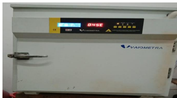
Photograph 3. Hot Air Oven (SDO-4554). Source. LOS, DOC, BBAU, Lucknow
