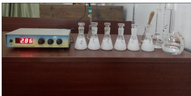
Photograph 5. Digital pH Meter (CL54+). Source. DOC, BBAU, Lucknow
