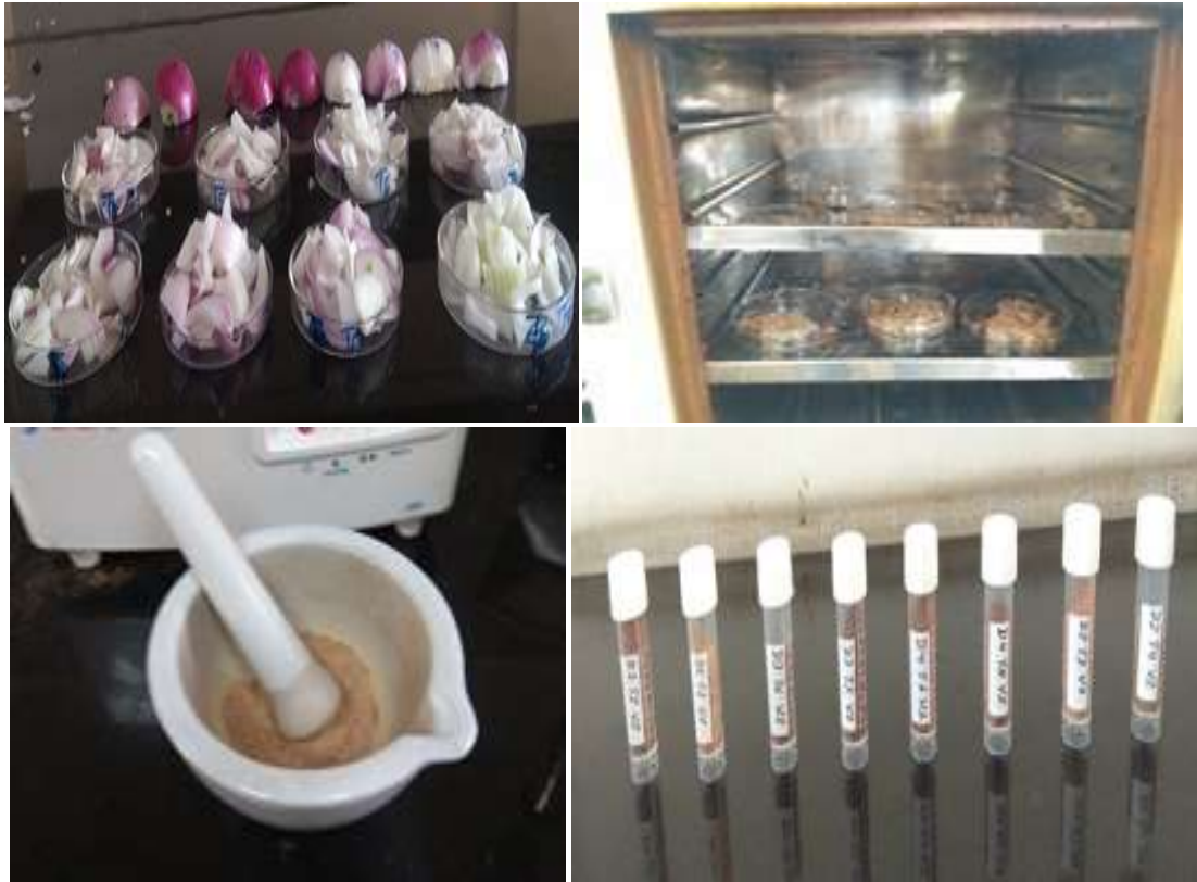
Plate 21: Sample preparation for determination of sulphur
