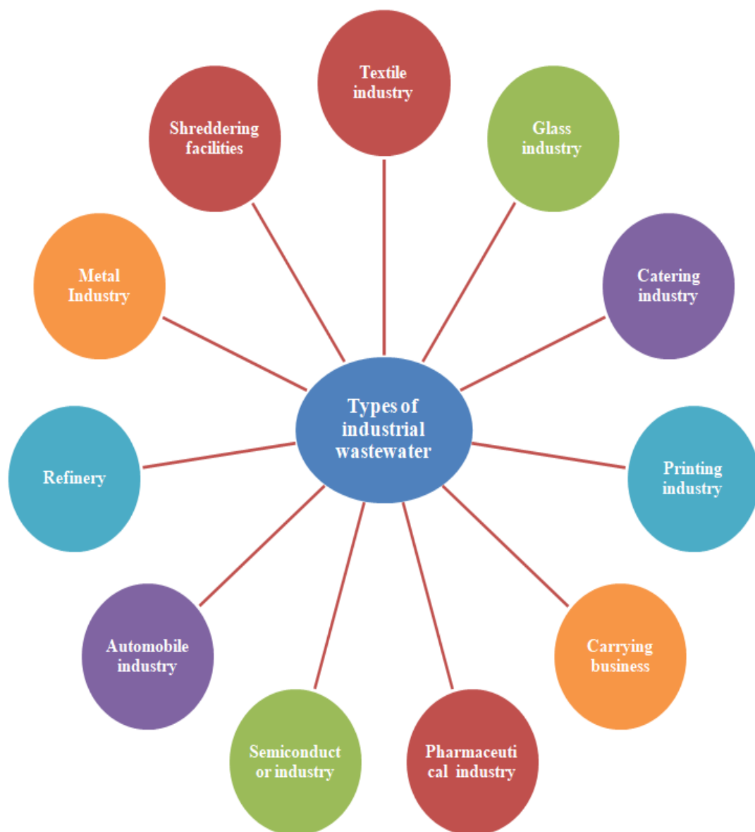
Figure 1.3: Types of industrial wastewater
