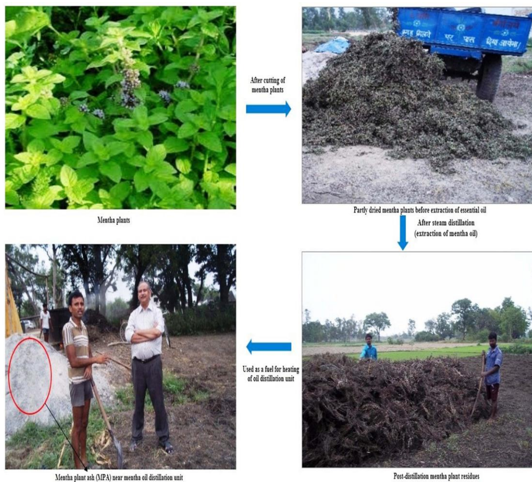
Fig. 3.2. A schematic diagram representing the generation of Mentha Plant Ash as a waste byproduct of mentha oil distillation unit.
