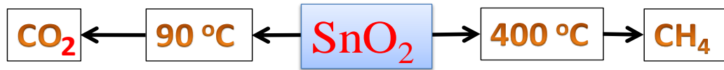
Fig. 1.2: A thermostatic cycle of a sensitive element (SnO 2 ) for CO 2 and CH 4
