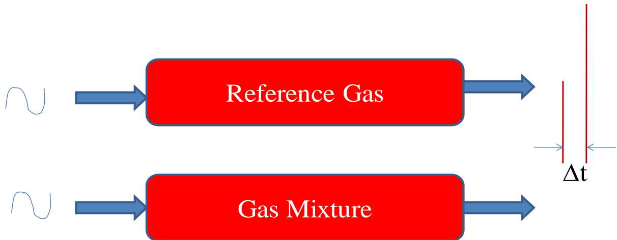
Fig. 1.3: Schematic of the method of ultrasonic detection
