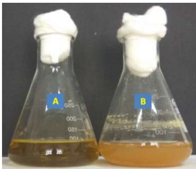
Fig. 8.2 Untreated (A) and treated TWW (B) by the newly developed bacterial consortium GS-TE1310
