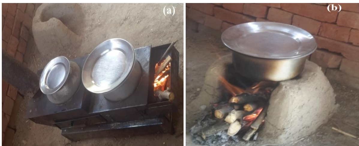
Figure 6.2. (a) Improved metal chulha (IMC), and (b) Traditional mud chulha (TMC) used in rural India.
