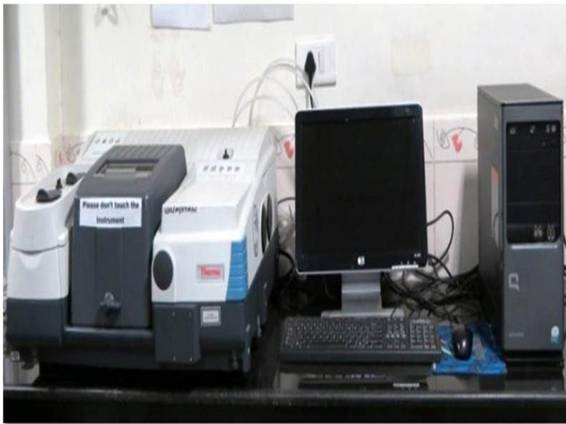
Figure 3.6 Fourier Transform Infra-Red Spectrometer, University Sophisticated Instrumentation Centre, Babasaheb Bhimrao Ambedkar University, Lucknow, UP, India
