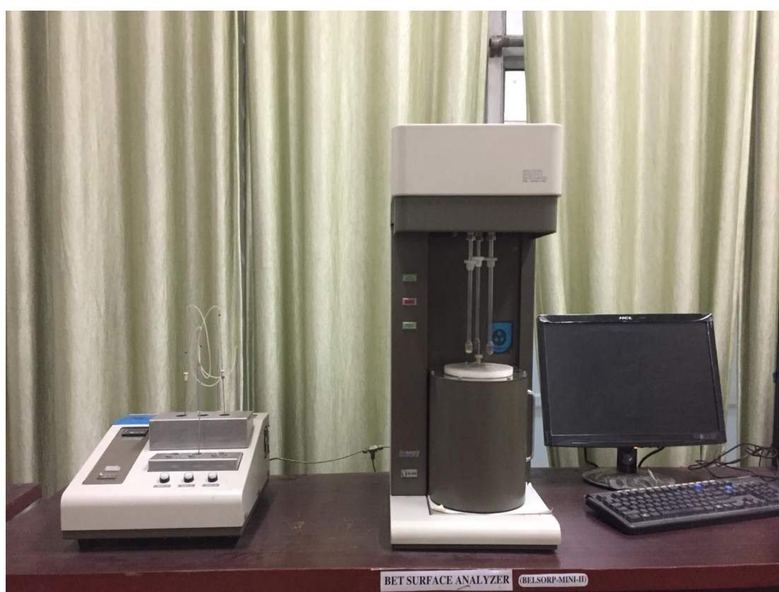
Figure 3.4 Brunauer Emmet Teller surface area analyser, Department of Chemistry, Babasaheb Bhimrao Ambedkar University, Lucknow, UP, India
