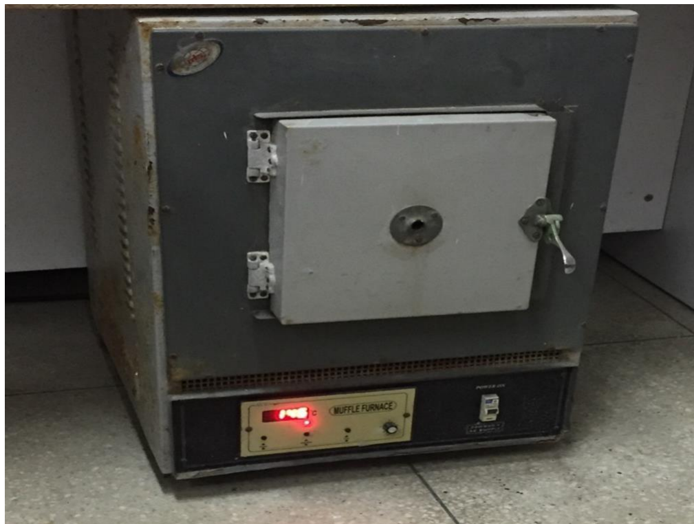
Figure 4.1 Muffle furnace for carbonization of bioadsorbents, Department of Chemistry, Babasaheb Bhimrao Ambedkar University, Lucknow, UP, India
