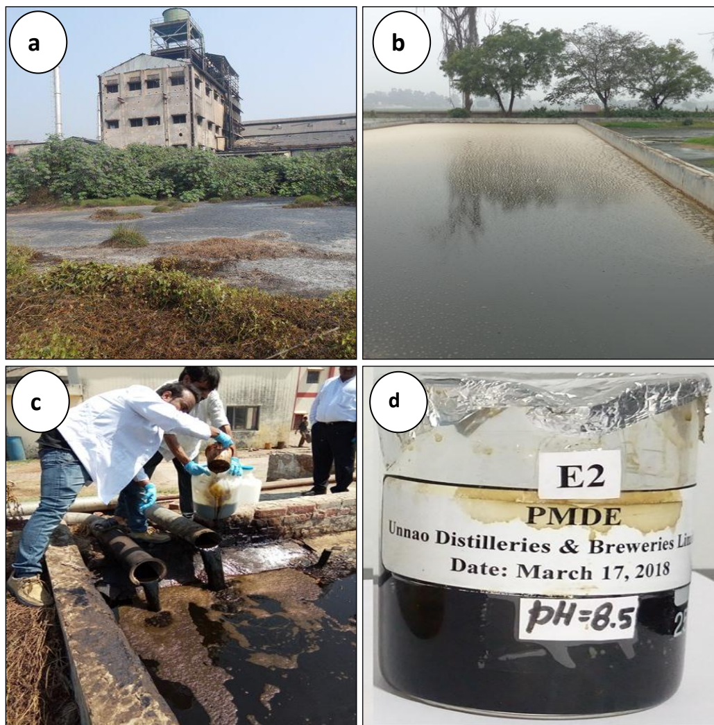
Fig.4.1. Sample collection. (a) View of M/s Unnao Distilleries and Breweries, Unnao (b) Post Methanated Distillery Effluent (PMDE) (c) Collecting PMDE (d) Collected PMDE
