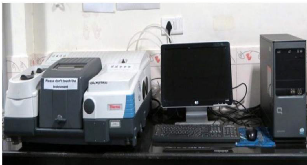
Fig. A.7 Experimental setup of FTIR: Thermo-Scientific Nicole 6700 (USIC, BBAU, Lucknow)
