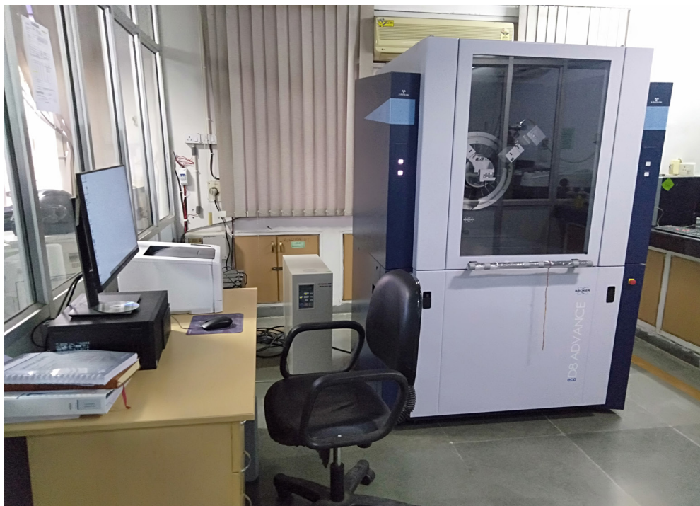
Fig. A.3 Experimental setup of XRD: Malvern Panalytical Ltd – X'Pert 3 Powder (USIC, BBAU, Lucknow)
