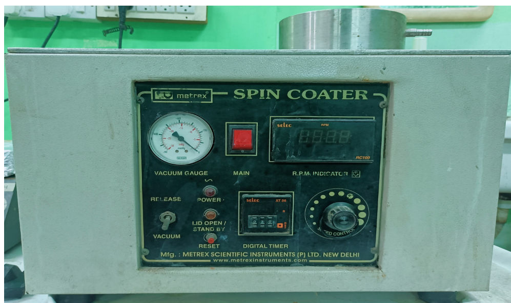
Fig. A.2 Experimental setup of spin coating: Matrex (NSRL, BBAU, Lucknow)
