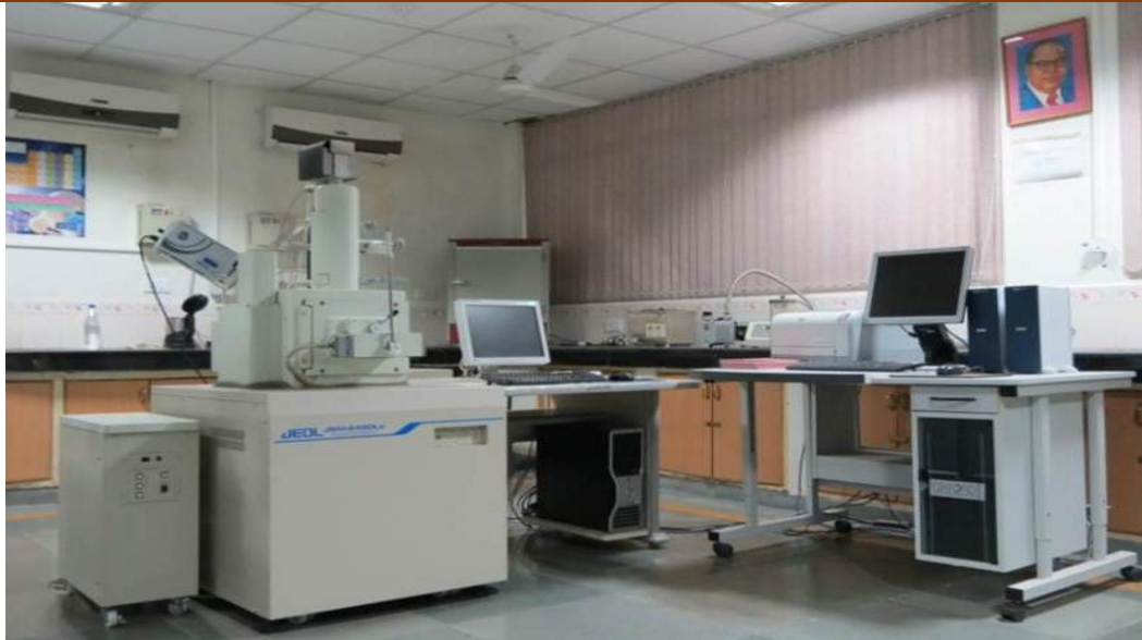
Fig.A.4 Experimental setup of SEM: JEOL JSM-6490 LV USIC, BBAU, Lucknow)
