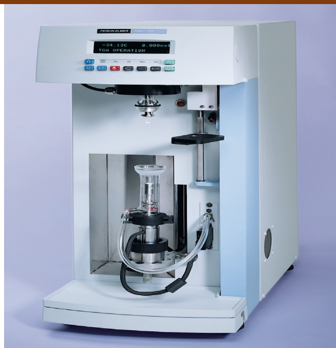
Fig.A.9 Experimental setup of TGA: Perkin Elmer Pyris 1 (CIPET, Lucknow)
