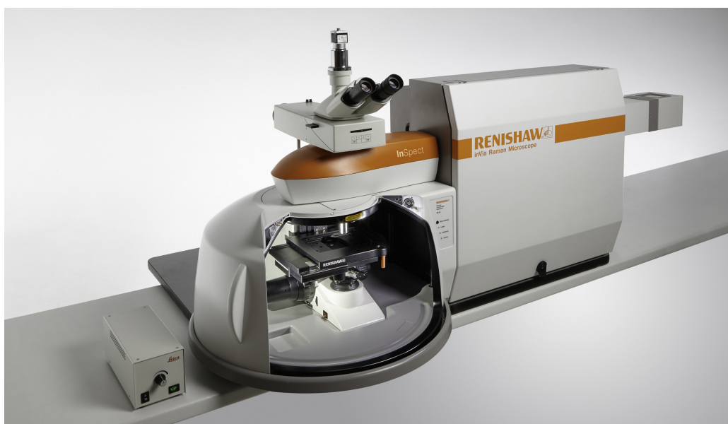
Fig. A.8 Experimental setup of RAMAN analysis: Renishaw inVia reflex micro-Raman spectrometer (CSIR-AMPRI, Bhopal)
