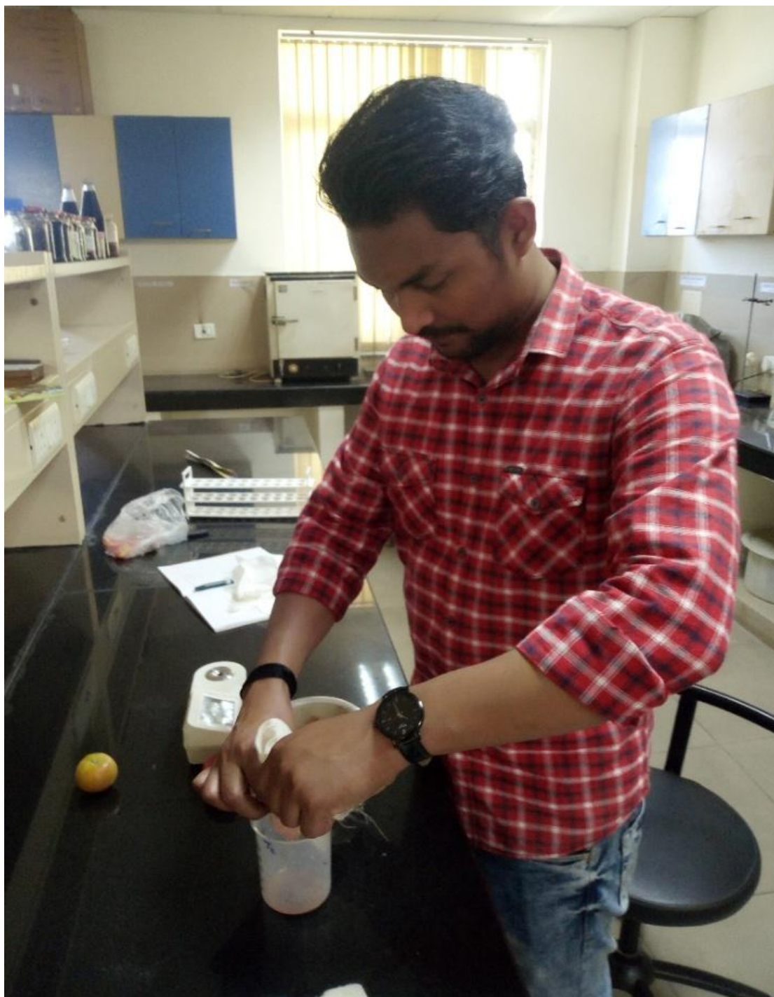
Plate-13: View of TSS ( 0 Brix) estimation in tomato fruit under laboratory condition.
