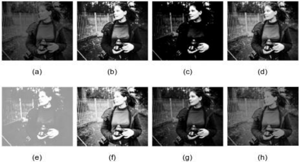
FIGURE 4.7 : (a) ORIGINAL IMAGE - 2, (b) Fuzzy IF-THEN, (c) Fuzzy Intensify Operator, (d) Fuzzy Histogram Hyperbolization (FHH), (e) FEV, (f) Contrast stretching (CT), (g) HE, (h) CLAHE
