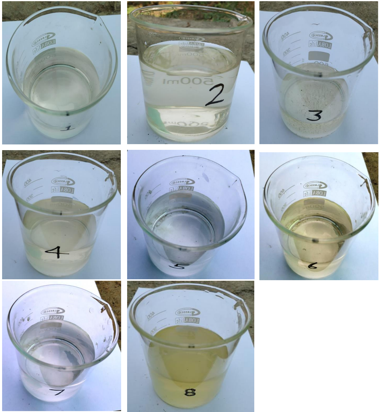
Fig. 3.6 Visual comparison of effluent quality between different treatment units. Number from 1 to 8 stands for Pi, Ph, T, Ph+T, Pi+Ph, Pi+T, Pi+Ph+T and Control unit respectively
