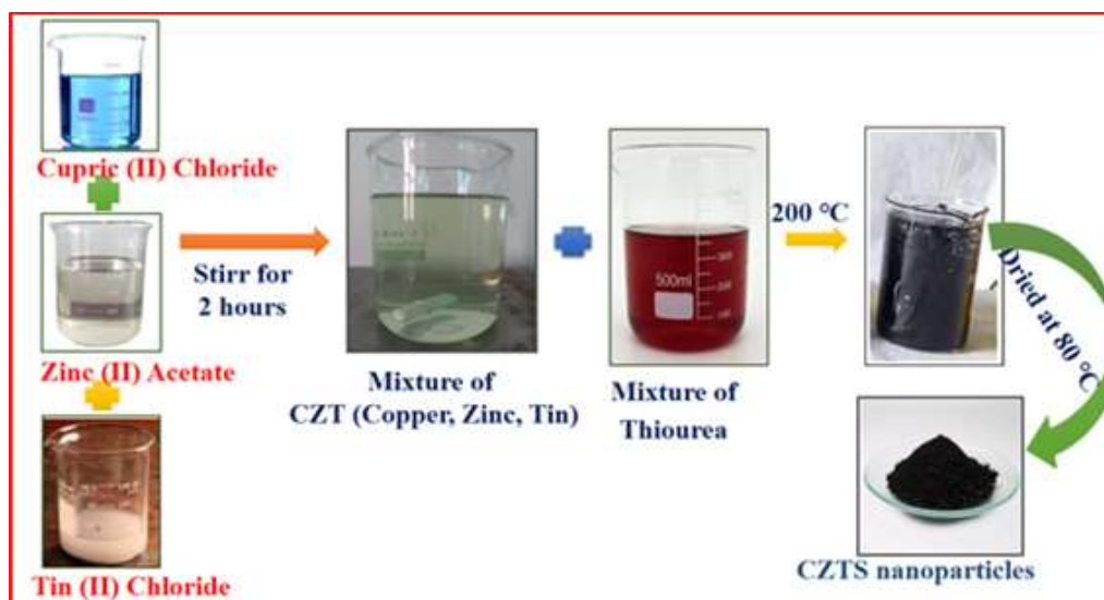
Figure 4.1: Schematic diagram for synthesis process of CZTS NCs by a chemical route.
