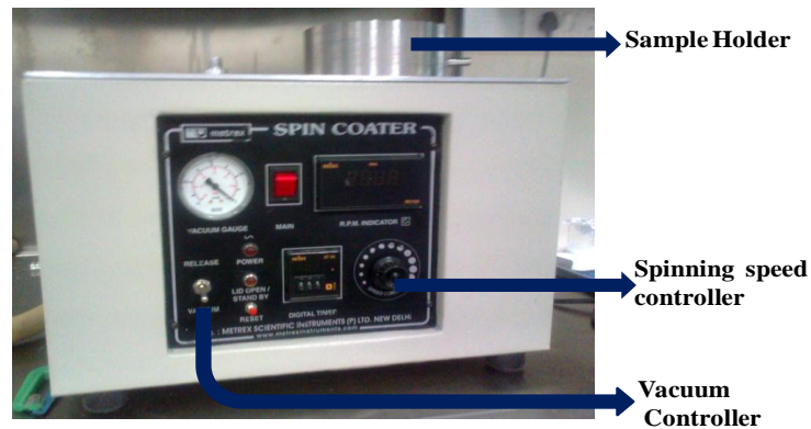
Figure A.2: Photograph of spin coater (Metrex) used in the preparation of thin film
