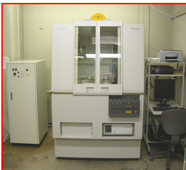
Figure A.5: Photograph of X-ray diffraction setup (X' Pert PRO PANalytical Ltd., Netherlands).
