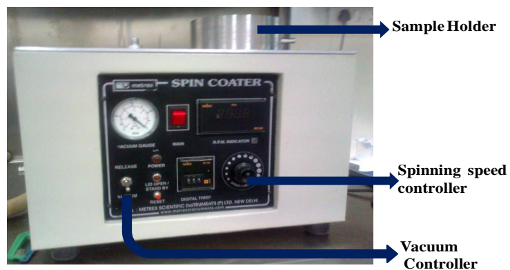
Fig. A.3: Photograph of spin coater (Metrex) used in the preparation of thin film.
