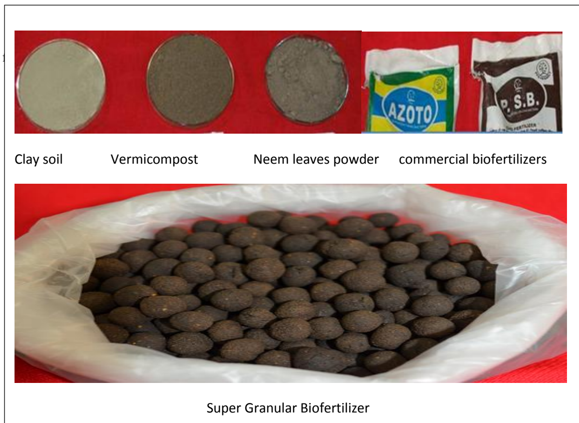
Plate: 3.1. Organic matrix such as clay soil, vermicompost, neem leaves immobilized with commercial charcoal based biofertilizers. Vermicompost is one of the best organic carriers among the FYM and cow dung
