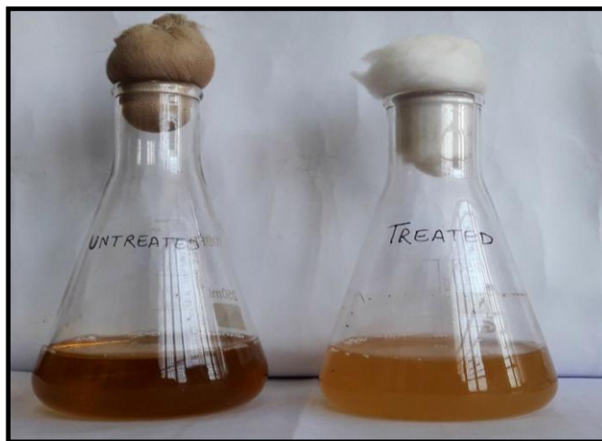
Figure 5.4: Degradation and decolorization of P&P effluent by a developed bacterial consortium of Bacillus aryabhatai (PLP 6), Bacillus megaterium (PNP 13) and Pseudomonas sp. (PNP 19).
