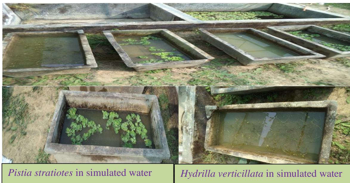
Plate 7.1. Showing the experiment conducted in the net house of DES, to evaluate the efficiency of selected plants for removal of nitrate, nitrite, ammonium and phosphate.
