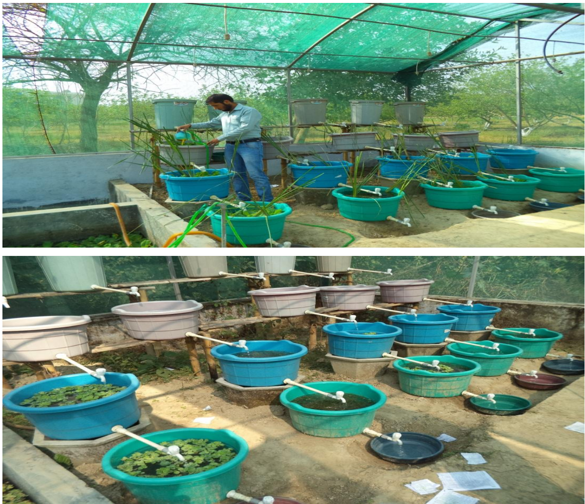
Plate 3.1. Plant based treatment system designed in NET House of Department
