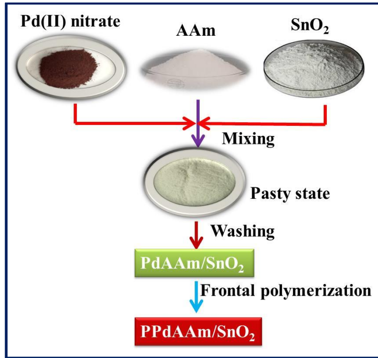
Fig. 5.1 Flowchart of synthesis of frontal polymerization of PdAAm@SnO 2 nanocomposite
