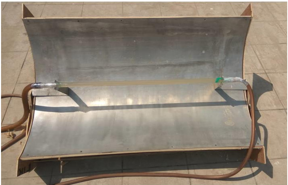
Fig. 3.5: (b) A pictorial diagram of PTR constructed for solar photocatalytic treatment of TWW.
