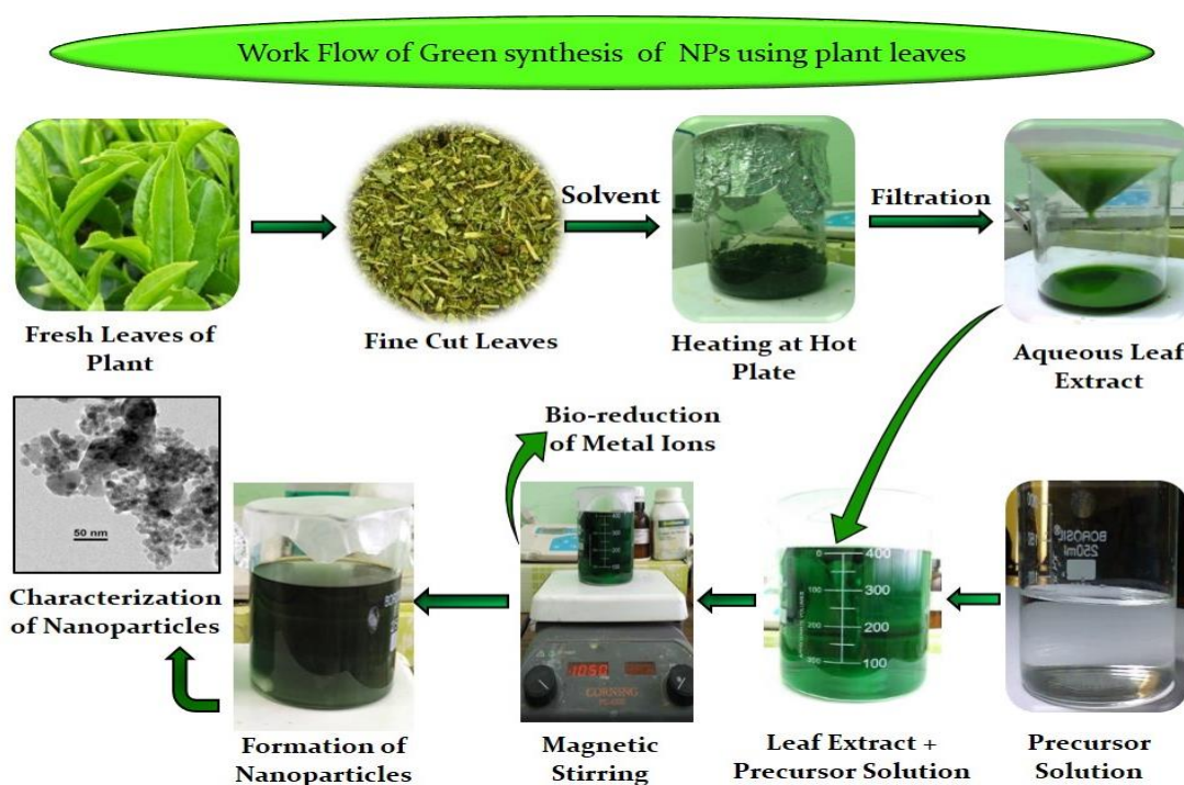
Fig. 1.2: The general process of green synthesis of nanomaterial using plant leaf
