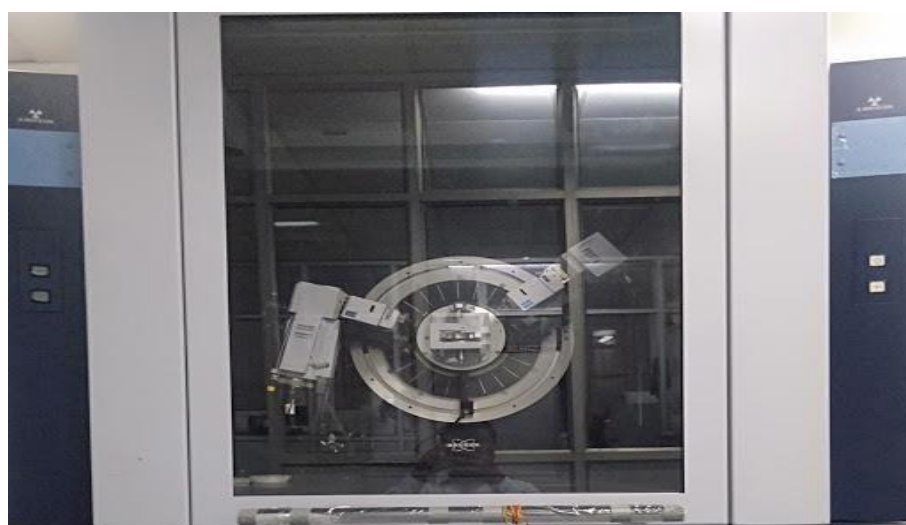
Fig. 3.6: X-ray Diffraction (Bruker ECOD8 ADVANCE), Source. USIC, BBAU, Lucknow
