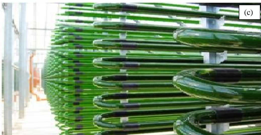
Fig. 1.3: Closed photobioreactor (a) flat panel photobioreactor; (b) vertical column photobioreactor; (c) tubular photobioreactor
